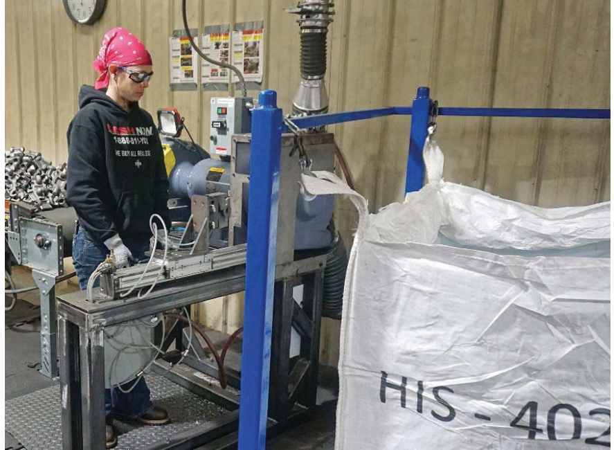
DONSCO process engineers tackle areas across the plant that can use optimization or automation, such as this finishing cell for trimming castings.
